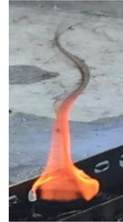
Fig. 2. Other fuel types (styrene based polymer) and smoke emissions which show the concept of incomplete combustion (shown to students by video safely); similar to room fires in real buildings.
